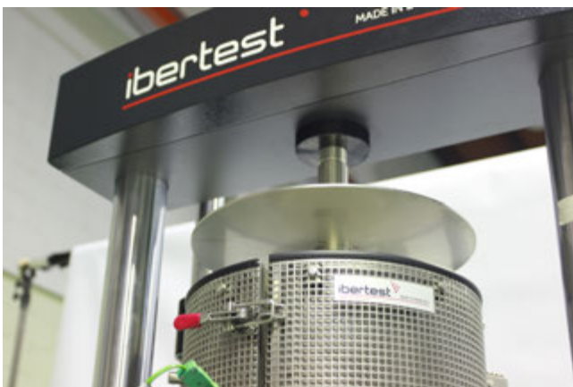
IB-CREEP-50 upper crosshead with spherical bearing and new furnace.
