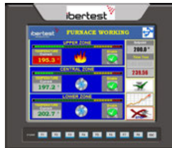
Testing Screen, 3 zones heating
