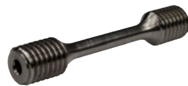
Typical steel specimen for creep test
