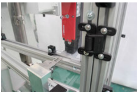
Safety cutout device in front main door - Outer and inner views
