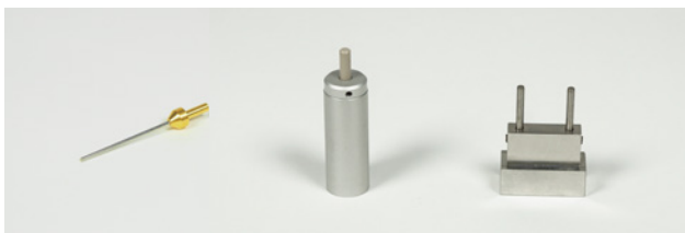
2 mm needle to ASTM C807 (63-L2700/F21) on the left; consistency probe and additional weight to ASTM C807 (63-L2700/F15) on the right
