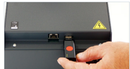
Communication ports are positioned on the rear side. LAN port is suitable for connecting to a PC or to LAN-hub, that creates a network with up to 32 independent units controlled by a single PC. USB port is used for data download to PC and firmware upgrade.
