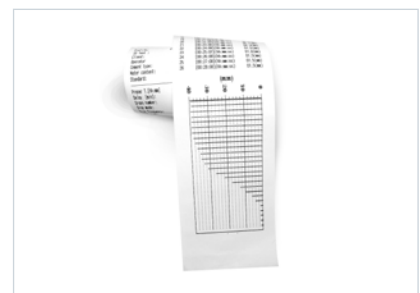
A typical plot of a test result obtained with the integrated printer model 65-L2700/E13 including setting time diagram and readings.
